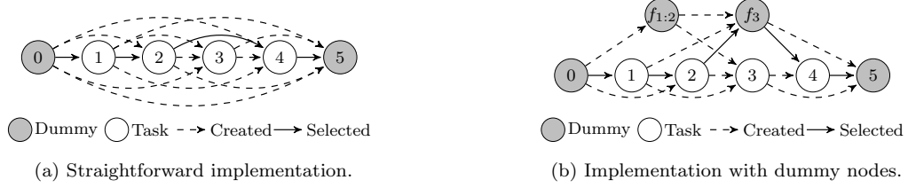
Figure 3: The same solution space of a 4-task instance represented on different graphs.
