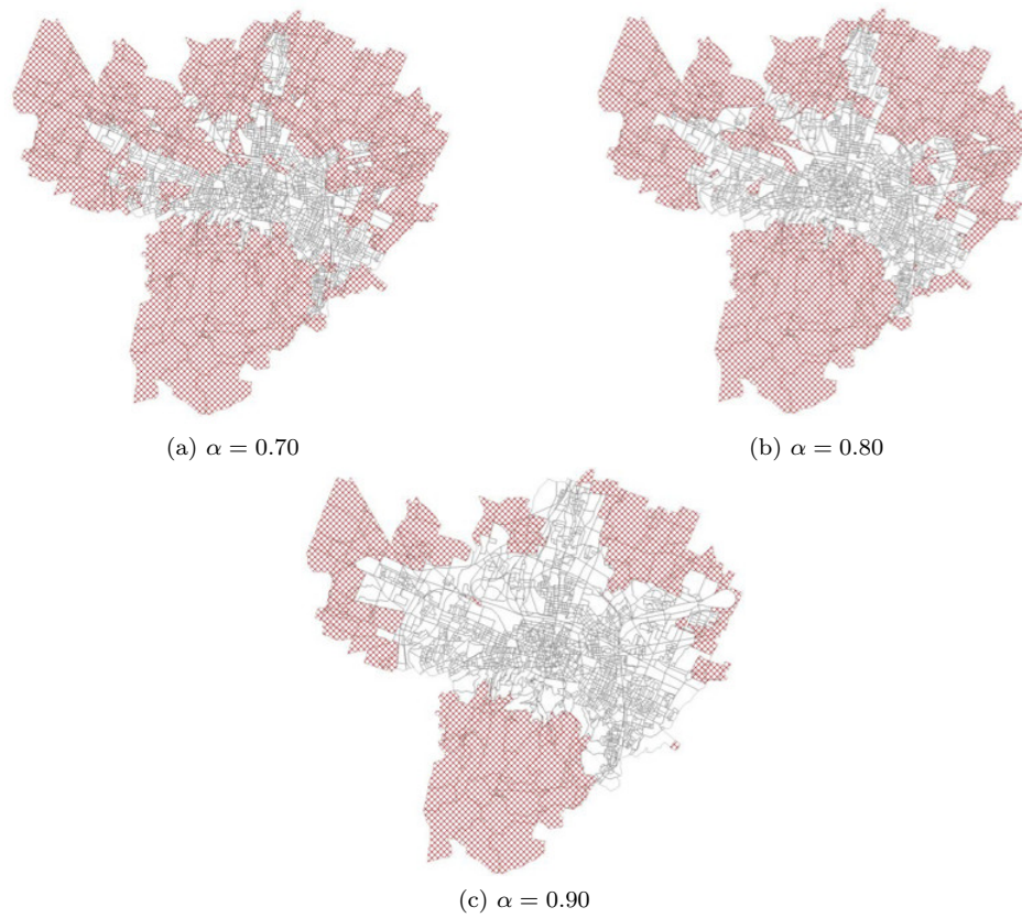
Figure 5. Partitioning of the users into a set I' of disadvantaged users (red) and a set I \setminus I' of non-disadvantaged users (white) by varying \alpha
